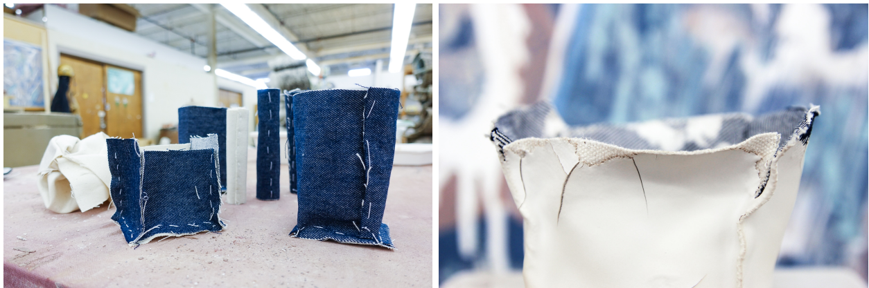
Figure 12: Hand-stitched 3D denim as scaffolds. Left: the denim scaffolds came in various forms to offer more freedom in design. Right: ceramic slip dried on the fabric scaffold before firing.
