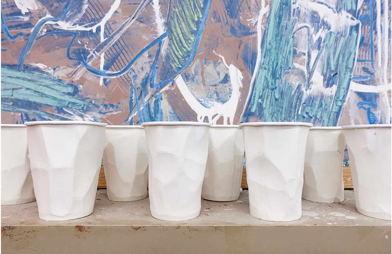
Figure 9: Result of experiment one. Drying slip left one-off polygonal imprints onto the cups.
