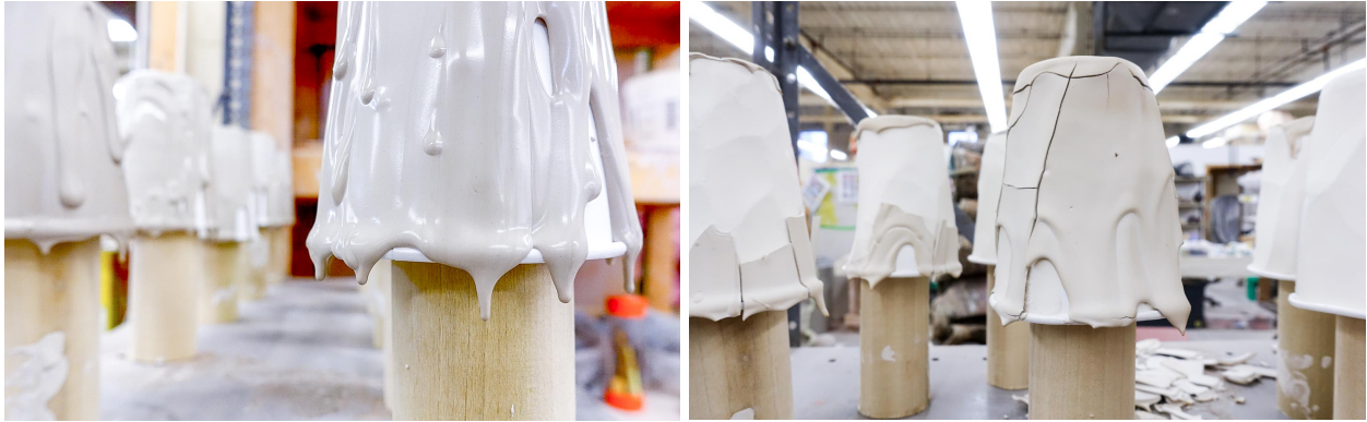
Figure 8: The making process of using paper cups (with a wax coating inside) as scaffolds. Left: ceramic slip took different forms during free dripping, depending on the weight and fluidity of the slip as well, as the humidity and temperature of the environment. Right: ceramic slip shrinks when it dries but the wax layer on the paper cups prevents the slip from shrinking: the pressure continued to accumulate and eventually cracked the slip, creating surprising polygonal imprints.
