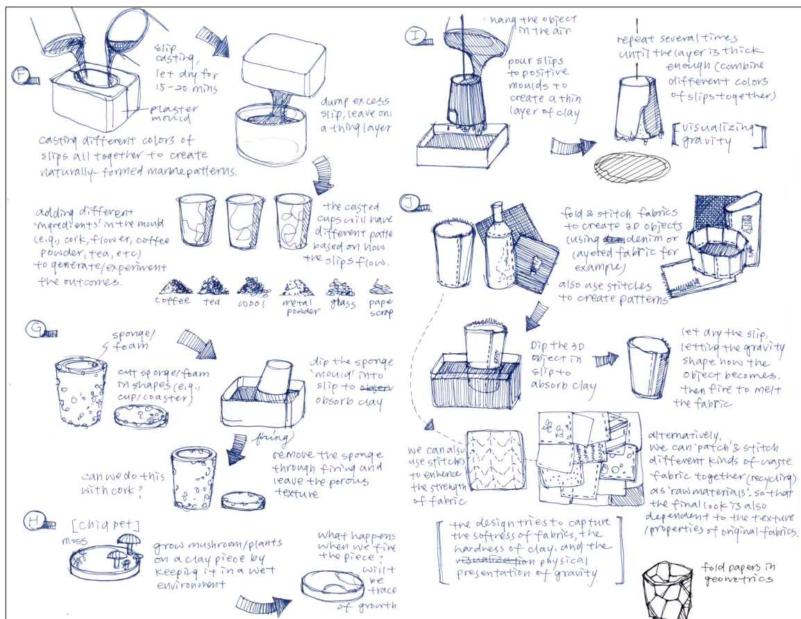
Figure 7: Ceramic experiment sketches. The ceramic making experiments aim to evaluate the four design tactics associated with scaffolding by implementing them in material forms.
